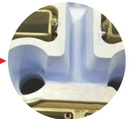
No Aluminum Adhesion Effect After 3 Casting Cycles
